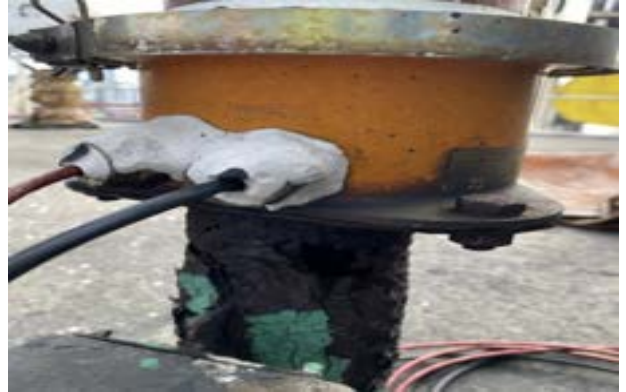
VDR mounting bracket on monkey island thinned, holed and wasted. [Not as required]
