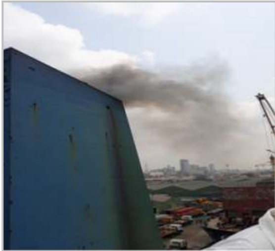
Excessive black smoke exhausting through funnel. (Air pollution) [Other]
